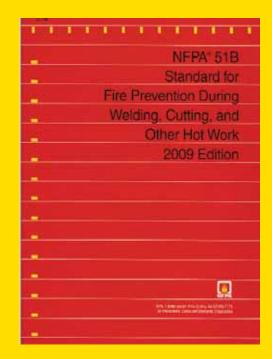
NFPA 51B (2009) now requires that welding blankets, curtains and pads be listed, approved or the equivalent for such use. One such listing includes ANSI/FM 4950. Many end users require adherence to the 2009 NFPA 51B Standard, thereby making hot work safer. The NFPA 51B Standard is most often cited by U.S. government agencies (OSHA, DOE) and private industry groups (API, AWS) for fire protection.
